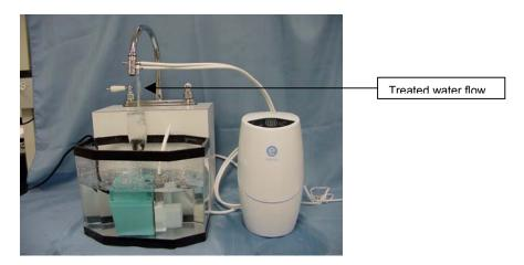
Looking at the back of the faucet and stand, the pump will be connected to the cold water faucet connection. The faucet cold water handle will need to be open when the pump is running and water is flowing. If there is a hand sprayer attachment, this will need to be detached and the connection plugged. The hot water connection will also need to be plugged.
