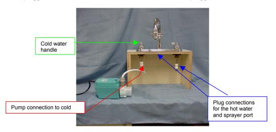
Connect the water pump to the cold water faucet with a piece of tubing. The tubing length must be long enough to connect to the pump when it is inside the water tank or aquarium.
